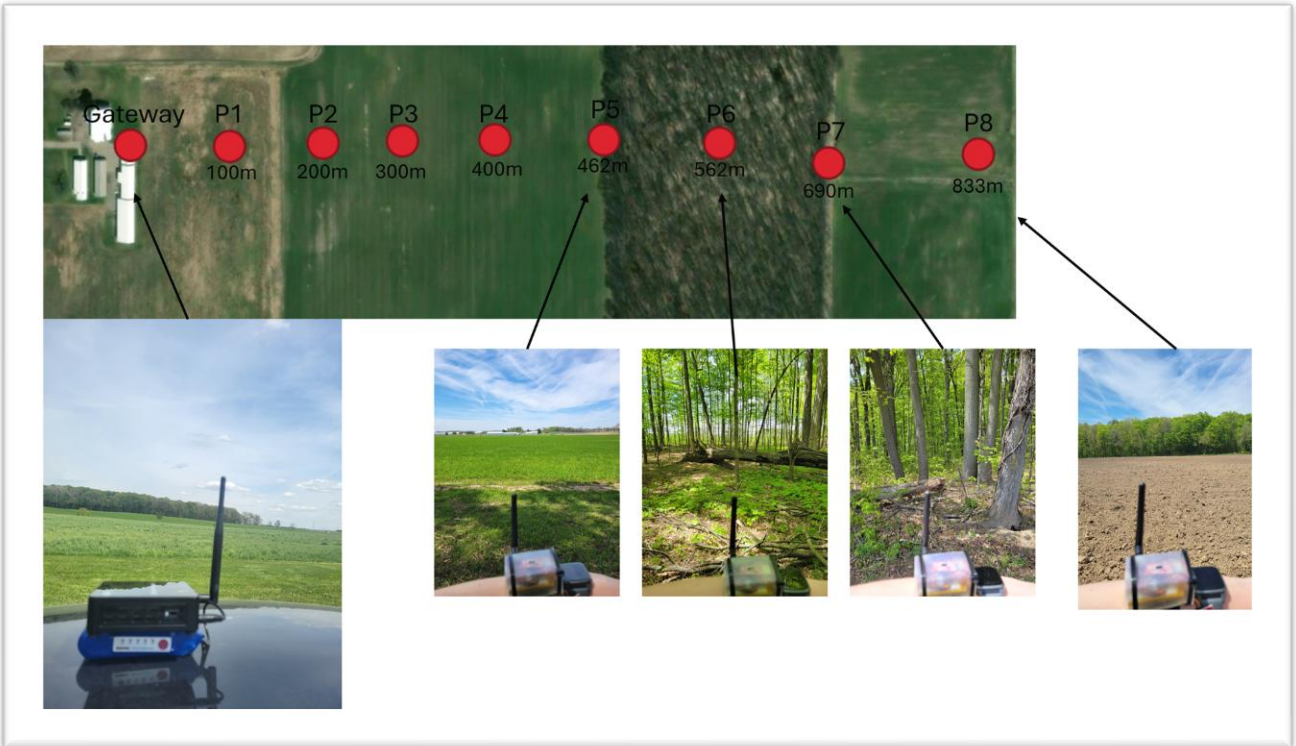
Figure 5: April 2 nd , 2026 mixed Terrain Test Path and Measurement Points. Test path showing progression from open field to dense vegetation, with the tree line at ~462 m. Measurement points indicate distances from the gateway.
